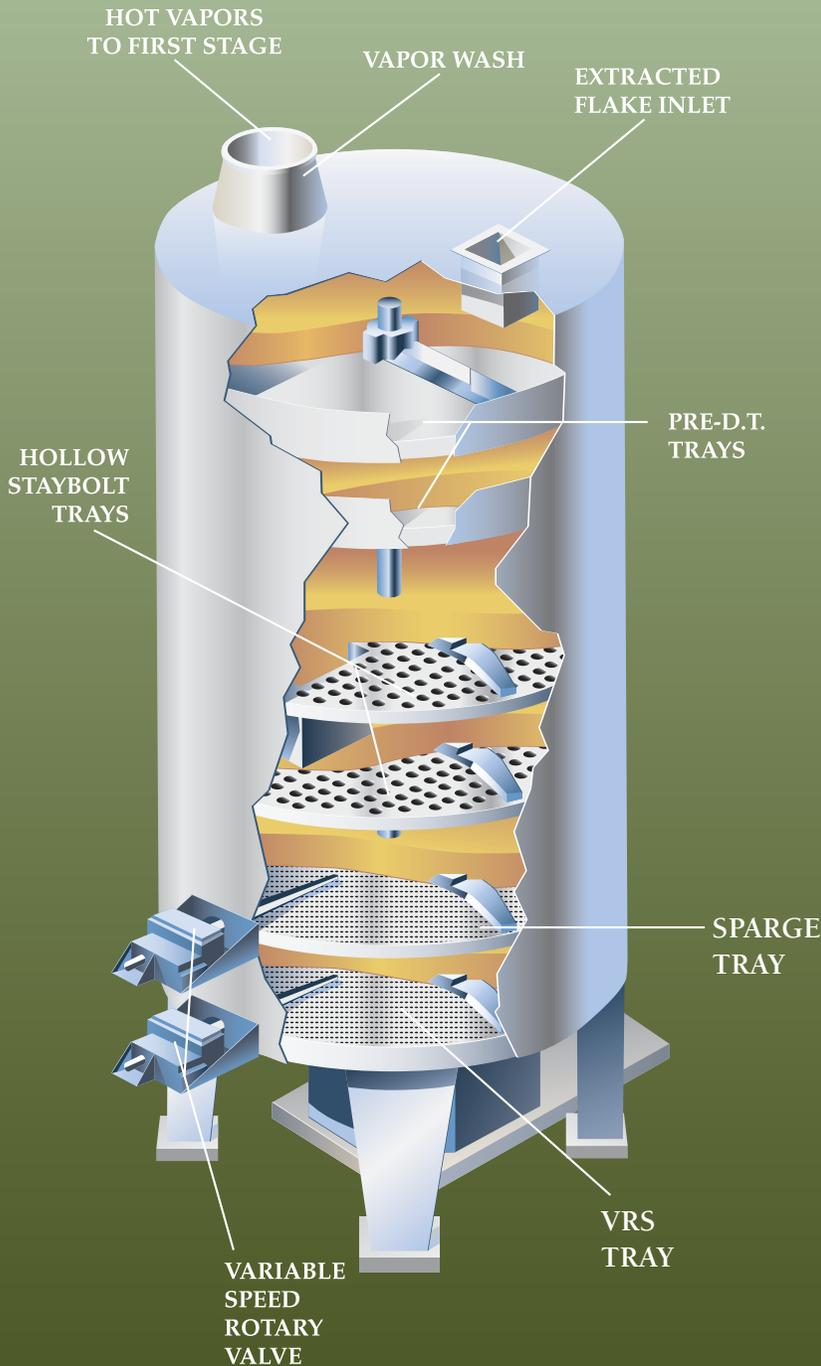
The VRS consists of an added tray below the sparge tray, preferably with a second rotary valve. This chamber is maintained just above ambient pressure to virtually eliminate leakage or flashing of steam from the outlet of the final rotary valve.
