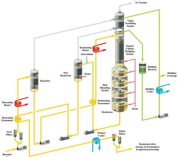
Maximum deodorizing efficiency with thinfilm stripping in packed column.
